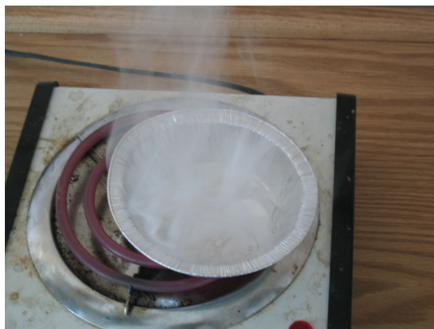
Figure 6. The setup for the 2000 mg “smoke” using the hot plate and an aluminum plate.
