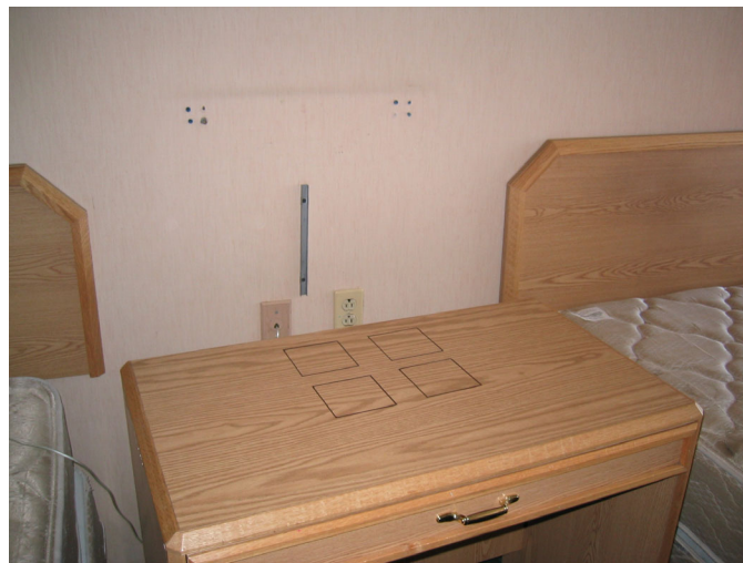
Figure 3. Horizontal wipe sample location D showing the 4 – 100 cm 2 sampling locations.
